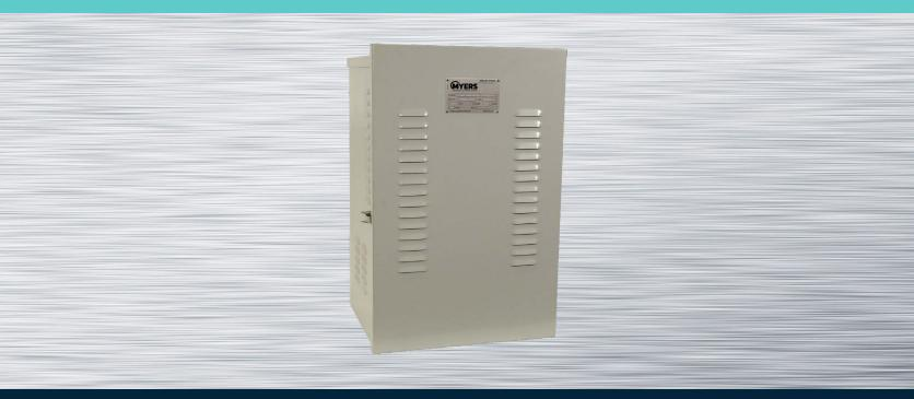
Pole or wall mounted outdoor rated enclosures for cable telecommunications and broadband applications. Accomodates one power supply/UPS with 0 to 8 Group 27 or 31 sized top terminal batteries. Includes: pole bracket, cable network, power interface with bypass switch, enclosure status LED, all cables to support /connect specified number of batteries. Optional:exhaust fan, breaker box and AC or DC generator interfaces.
