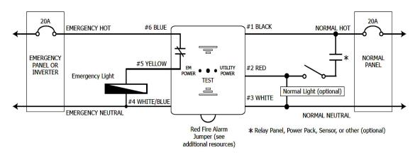
Note: Emergency light is also called N/E light or Normal/Emergency light by many specificiers
