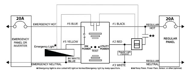
Note: Please refer to RLY-INT/CTRL-2 installation instructions for inverter interface wiring diagram.
