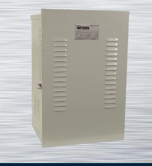
Pole or wall mounted outdoor rated enclosures for cable telecommunications and broadband applications. Accomodates one power supply/UPS with 0 to 8 Group 27 or 31 sized top terminal batteries. Includes: pole bracket, cable network, power interface with bypass switch, enclosure status LED, all cables to support /connect specified number of batteries. Optional:exhaust fan, breaker box and AC or DC generator interfaces.
