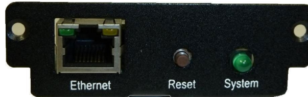
Figure 6-39: Ethernet-to-Serial Adapter Card Front Panel.
