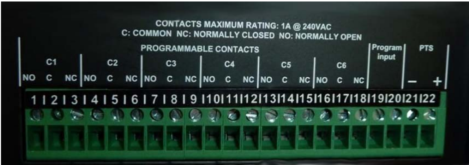
Figure 2-6: MP2000E Battery Backup System Control Terminal Block
