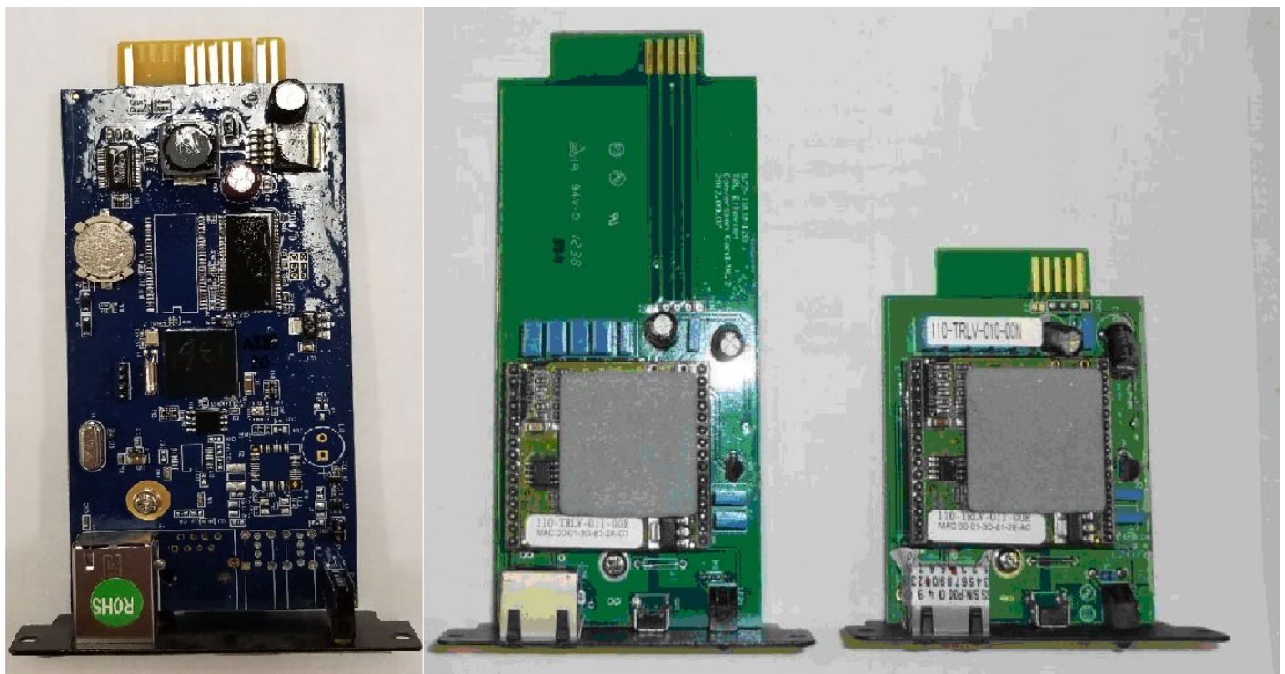
Figure 6-40: HTML Ethernet and Ethernet-to-Serial Adapter Card Interior Views
