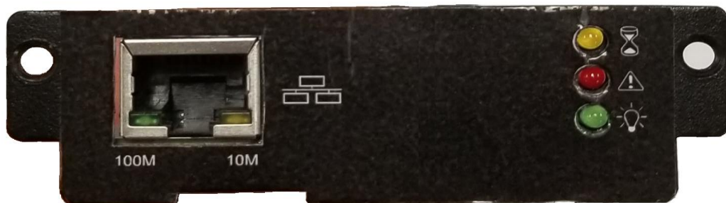
Figure 6-38: NetAgent Embedded HTML Ethernet Card Front Panel
